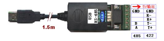
USB485 is an 1.5 meter long wire including USB port and RS-485/422terminals. The drive software is in a CD-ROM and it is the same as BOSI USB232. How to intsall the driving software"
