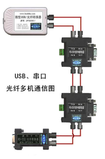
Note: the TX1 and RX1 to up direction, TX2 and RX2 to down direction.
